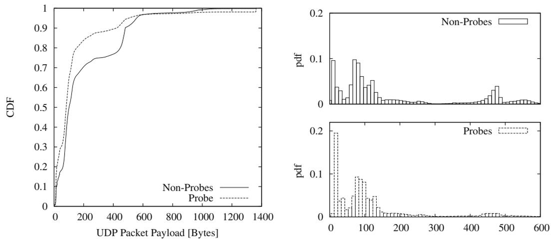
Fig. 5. Probe versus non-probe traffic packet size.
