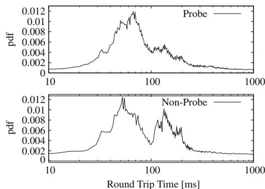
Fig. 8. Probe versus non-probe traffic: round-trip times.
