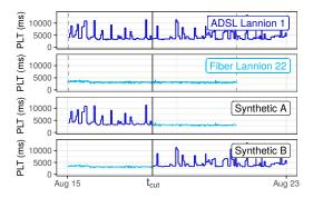
Fig. 2: Quasi-experimental methodology for building a synthetic network ground truth. Given a pair of time series (top), two synthetic series are computed (bottom). Solid black line indicates  $t_{cut}$ , dashed gray lines correspond to the [a, b] range.
