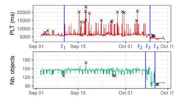
Fig. 1: Example time series from our dataset: Page Load Time (top) and number of objects in the page (bottom) in *http://lefigaro.fr* website. Vertical annotations (blue lines) are obtained with change point algorithms described later in this paper. For the sake of illustration, we mark with crosses outliers that deviate over  $3\sigma$  in each interval.
