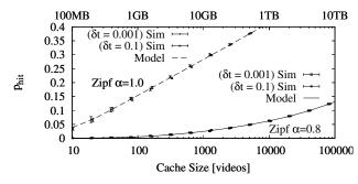
Fig. 2. Hit probabilities obtained by analysis and simulation for chunk interarrival time  $\delta t = \{0.001, 0.1\}$ , catalog size  $M = 10^8$ , Zipf  $\alpha = \{0.8, 1\}$ .
