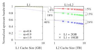
Fig. 3. Comparison between the performance of a standard cache and our two-layer cache: Normalized bandwidth in the (a) current and (b) future scenarios.
