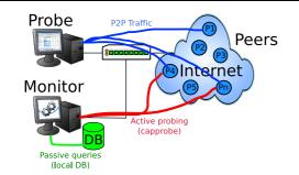
Fig. 6 P2PGauge analysis process
