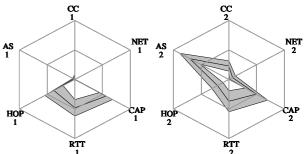
Fig. 8 Network-awareness representation: Kiviat charts of (a) Preferential partitioning and (b) Kullback-Leibner divergence on the new SopCast dataset. Features gathered with passive measurement are displayed on top axis (AS, CC, NET), features requiring active measurement on the bottom axis (HOP, RTT, CAP).
