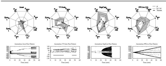
Fig. 5 Misbehaving and malfunctioning applications: Kiviat representation of average and anomalous endpoint behavior (top) and corresponding traffic level pattern of the anomalous endpoint (bottom) for P2P-TV and P2P-VoD applications.
